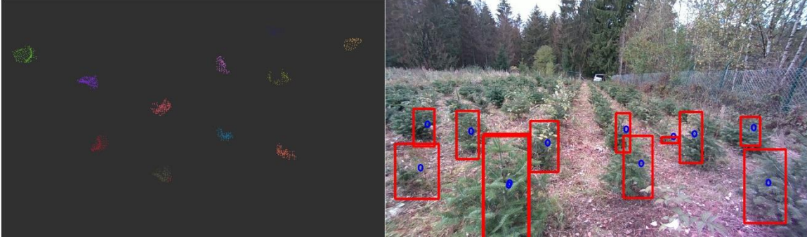
Figure 3: On the left you can see the point cloud clusters found in different colors from a bird's eye view. The image on the right shows the bounding boxes resulting from the clusters from a vehicle perspective.
