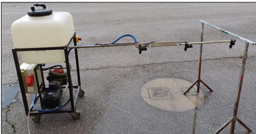
Figure 6. Experiment platform for valve and nozzle test.
