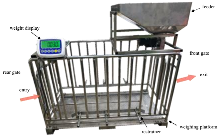
Figure 2. Image of the individual data collection system for pigs
