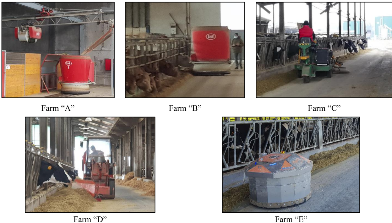
Figure 2. The feed-pushing machinery in the five farms under analysis: automatic feeding systems (Farm A, B), operator-based feed pushing (Farm C, D), automatic drum feed pushing (Farm E).
