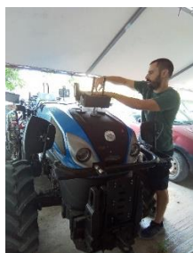
Adjusting perception unit for field test
