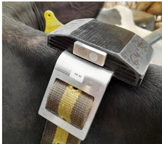
Figure 1: Sensor on the collar of a cow.
