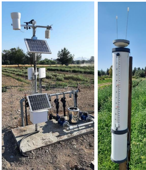
Figure.1: Automatic weather station and electronic atmometer connected to the station data logger unit.
