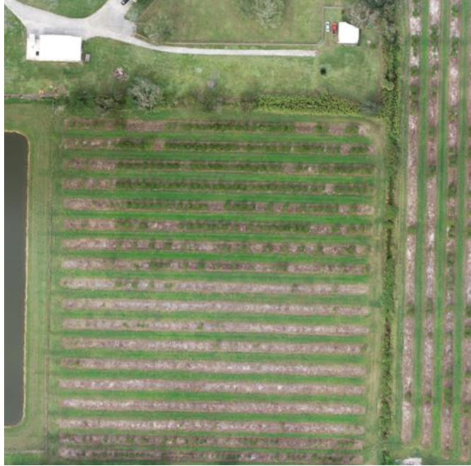
Figure 4. Orthomosaic map generated by Pix4D using GAN generated images.
