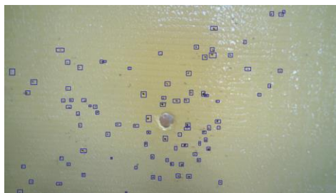
Figure 2. Example of an acquired image from the trap with bounding boxes enclosing the insects [19].
