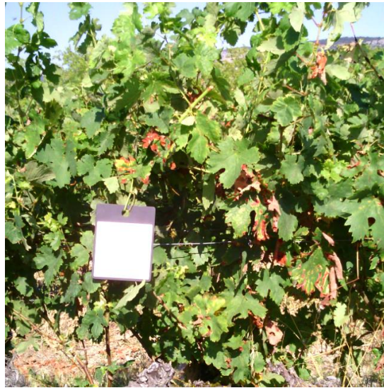
Figure 1. Picture of a vine taken in the field with the Spectralon plate (white reference).
