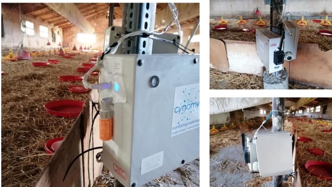
Figure 1. uRADMonitorA3 (right) and cynomys sensor systems (left) placed in the broiler house.
