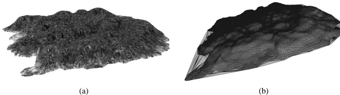
Figure 3. An example of (a) point cloud and (b) mesh creation for 3 kilogram feed, captured from 1 m at morning light.
