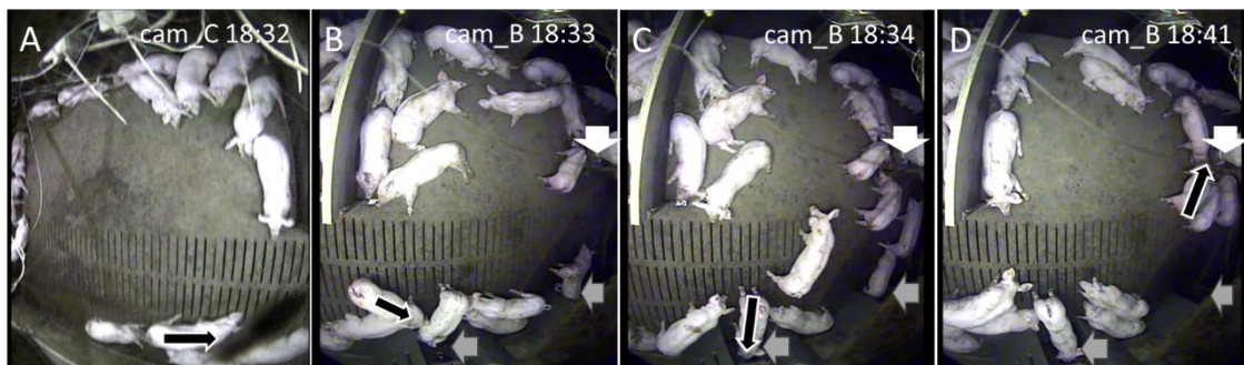
Figure 8: Screenshots illustrating manual verification of the track of pig 109 on 8/3/2015 showing the pig (A, black and white arrow) on camera (cam_C, A) moving into the area visualized by camera (cam_B, B) identified when drinking (C) and identified while eating (D). Images show the drinkers (grey arrows) and feeding station (white arrows) where HF RFID identification can be performed in the area visualised by cam6.
