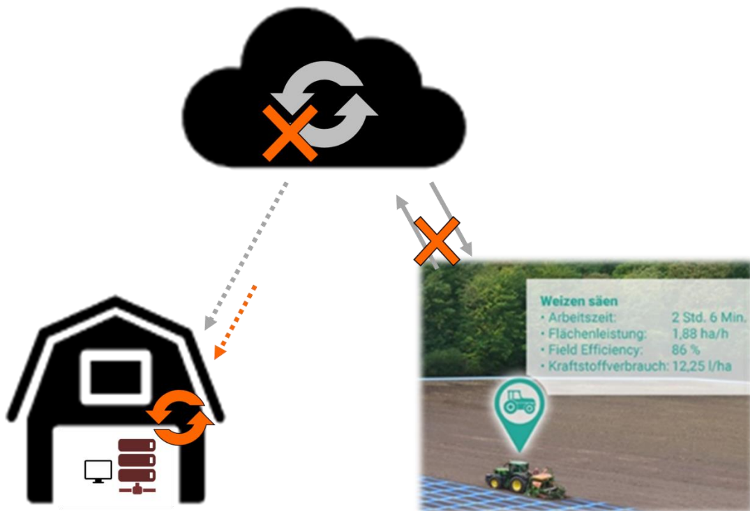
Figure 1: The grey symbols represent the regular way of communication and prediction by AI. In case of interrupted communication, the farm server continues automatically the same prediction procedure with the latest machine data. (Translation of picture descriptions: Weed seeding; working time: 2h 6min, area output: 1.88 ha/h, field efficiency: 86%, fuel consumption: 12,25 l/ha)
