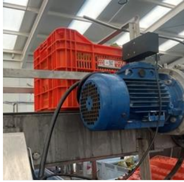
Figure 4 - Automated box scanner employed during the grape reception phase at wineries.
