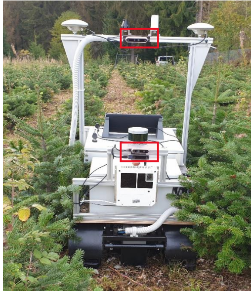
Figure 2. Robot equipped with various sensors, including two RGBD (red frame) cameras.
