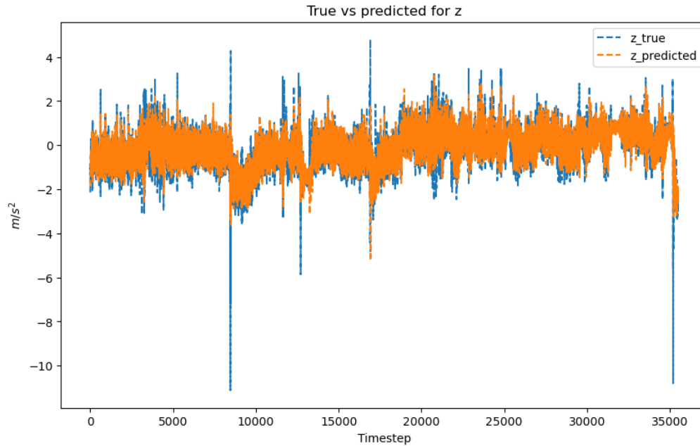
Figure 3. Results for the z-axis when applying the Autoformer model to one hour of the dataset.
