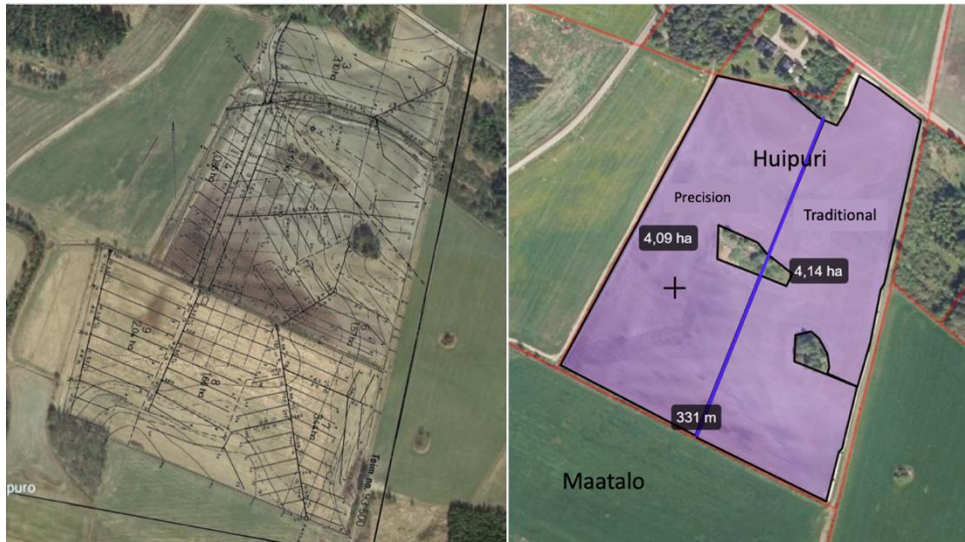
Figure 2. Test Plots. On the left, a drainage map; on the right, the division of the Huipuri field for precision farming and traditional cultivation.
