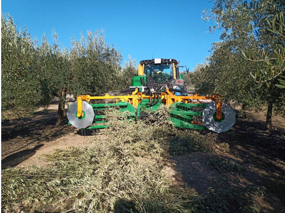
Figure 4. The prototype windrowing, chipping and harvesting olive biomass during field tests.
