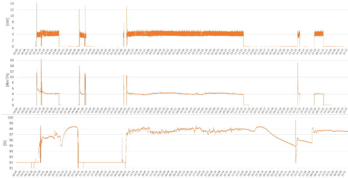
Figure 11. BioCNG plant power consumption (top), BioCNG flow rate (middle), and CH4 concentration of BioCNG (bottom) at the LVAT pilot farm.
