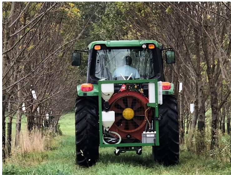
Figure 4. The in-line injection and mixing system attached to a laser-guided variable-rate orchard sprayer for field tests.
