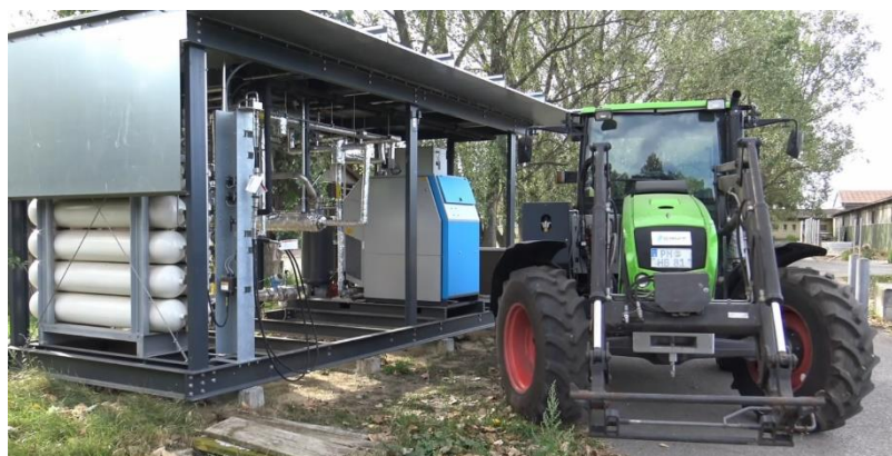
Figure 4. The Bio-CNG plant and filling station (left) and the biomethane tractor at the LVAT farm.
