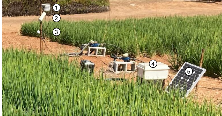
Figure 1. Image of the experimental plot. 1: ATMOS 14 sensor, 2: IR120 sensor, 3: SRS-NDVI field stop sensor, 4: CR1000 data logger protective box, 5: solar panel.
