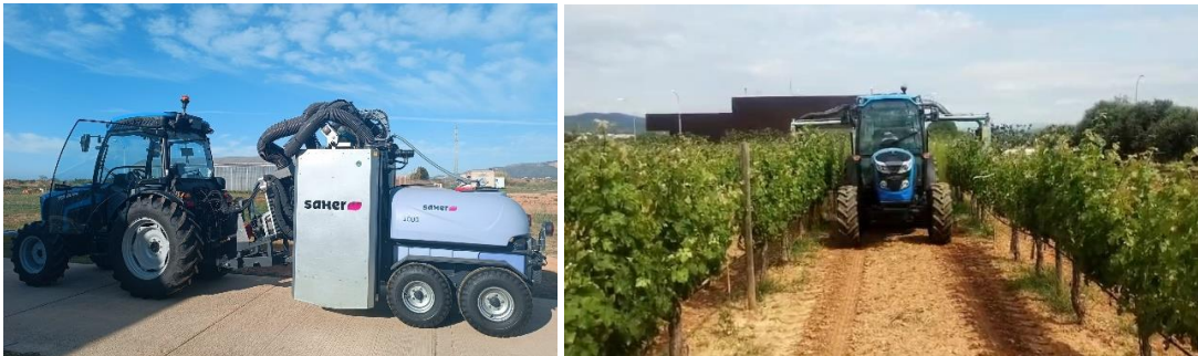
Figure 1. General schematic view of the experimental tunnel sprayer (left) and use of recovery panels during a spray application (right).
