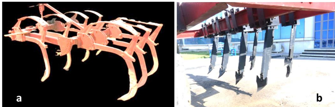
Figure 1: Main features and construction of chisel plows used (a) traditional plow (b) developed plow
