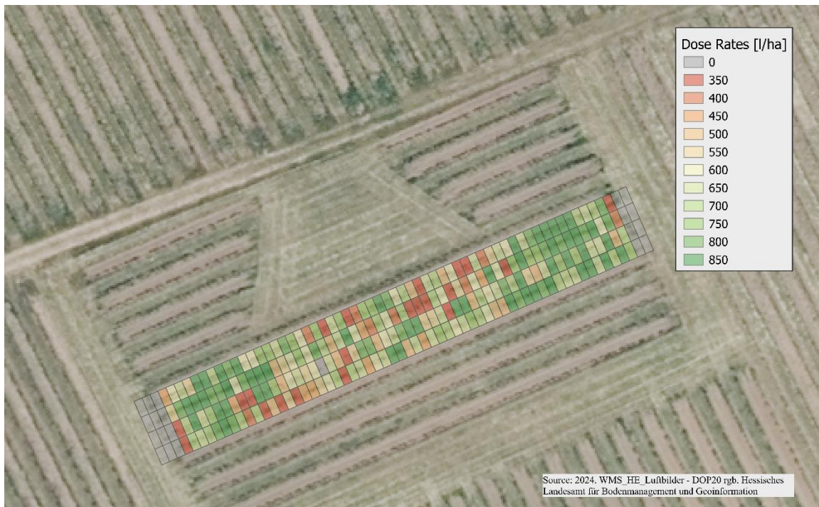
Figure 5. Prescription map with 1 x 2 m grids and leaf area adapted dose rates
