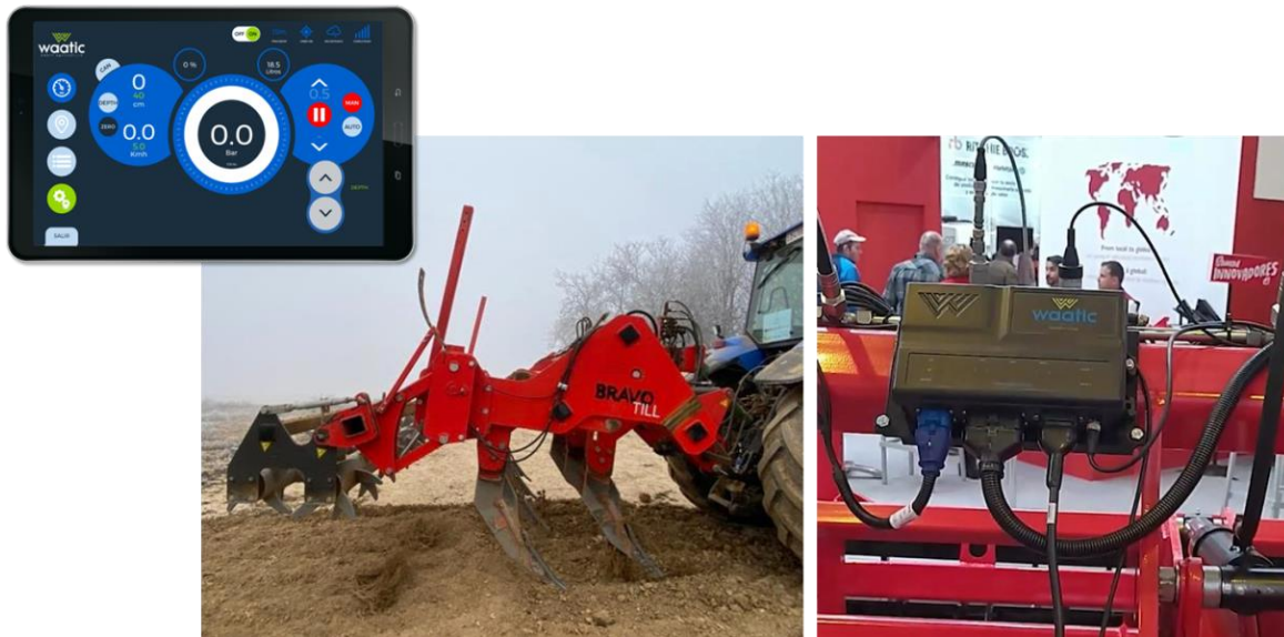
Figure 2. Detail of the soil resistance monitoring prototype developed, the control unit and the user interface
